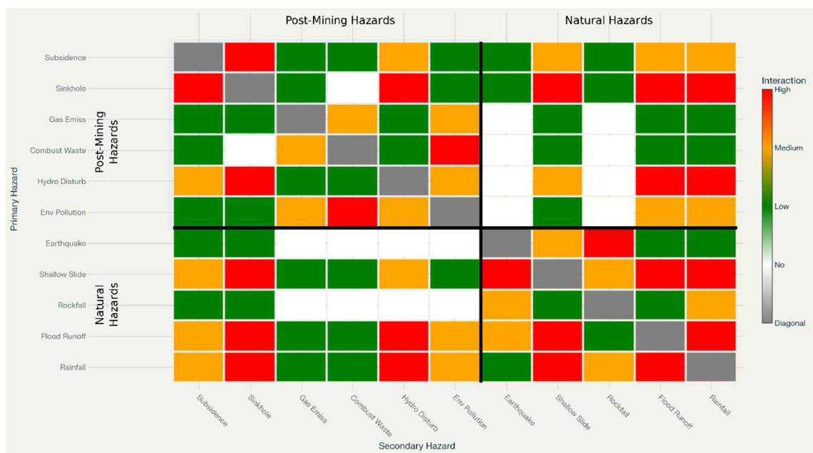
Figure 21: Interaction matrix for the Ruhr Area case study incorporating post-mining and natural hazards
